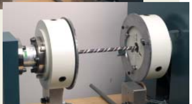
Fig. 3, 4 and 5. Test in progress on the 10,000 in.lbf model with a painted sample rod of steel.
