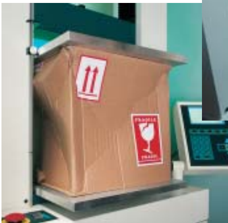
Fig 4. Direct compression test to determine the strength of cardboard packaging.
