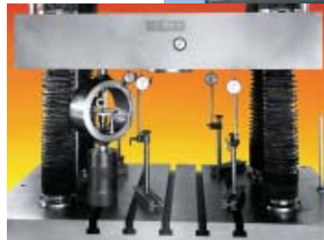
Fig 19. Proving ring and height indicator verify the off-center accuracy of four screw Electomatic with no appreciable eccentric movement of cross-head. Shown with optional tee slotted table.
