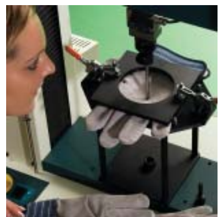
Fig 7. Puncture jig being used to determine the puncture resistance of work gloves.
