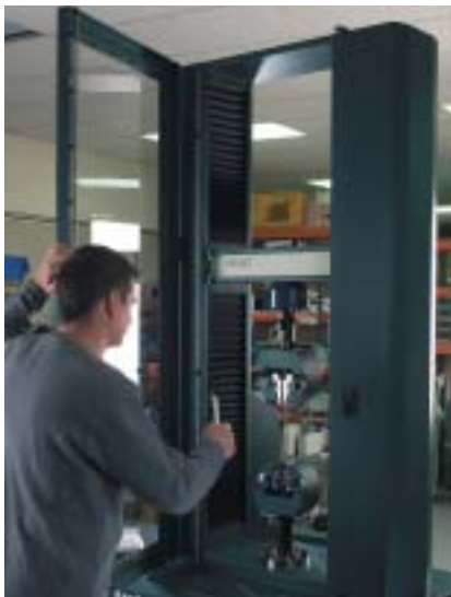
Fig 12: Model H100kT shown with interlocking safety door.
