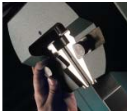
Fig 13. Close-up of HW21 grips being used on H100kT machine.
