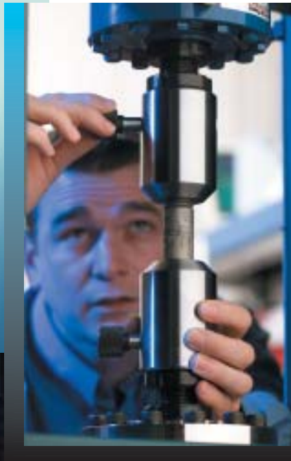
Fig 9. Test of a butt-welded part using threaded grips.
