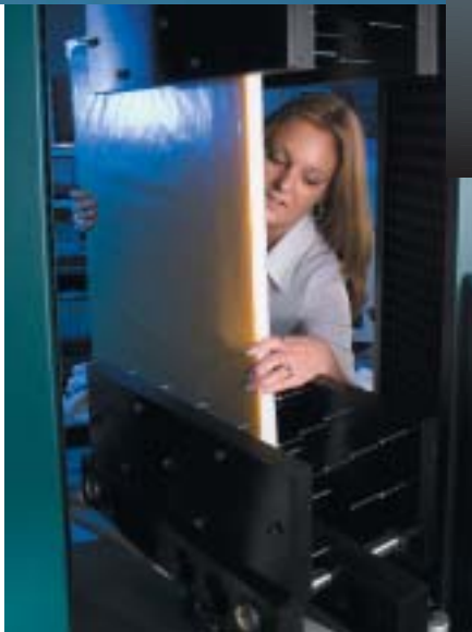
Fig 11. Model H100kT being used to test large sections of insulation board.
