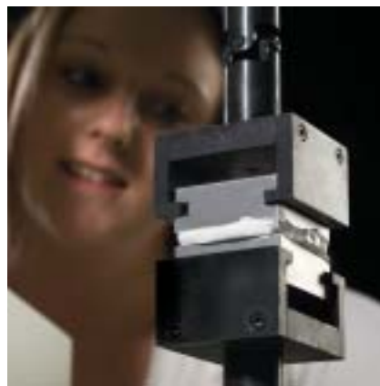
Fig 6. Claw adaptors being used to test the strength of adhesive/sealants.
