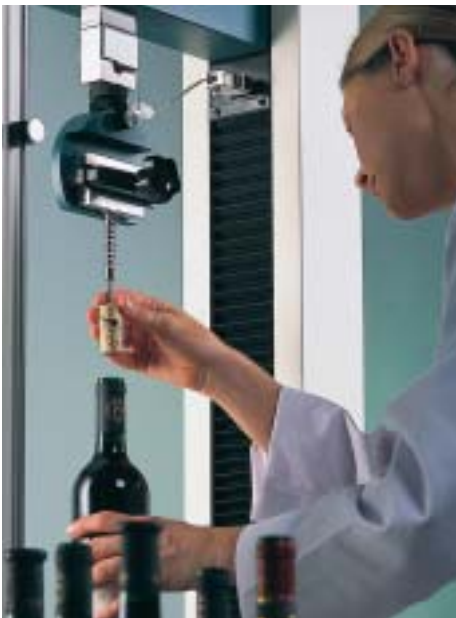
Fig 5. Tests involving the extraction of new corks from wine bottles. This application is testing new “cork” material.
