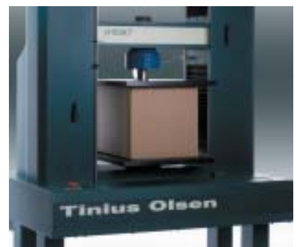
Fig 14. Model H100kT performing a compression test.
