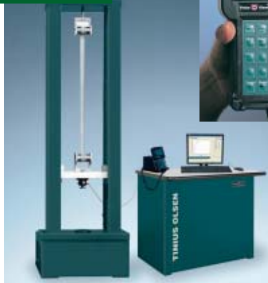
Fig 15. For testing high elongation materials or unusually long test specimens, Tinius Olsen can provide LoCaps with extended vertical clearances. This unit features an 8 ft vertical clearance (less tooling).
