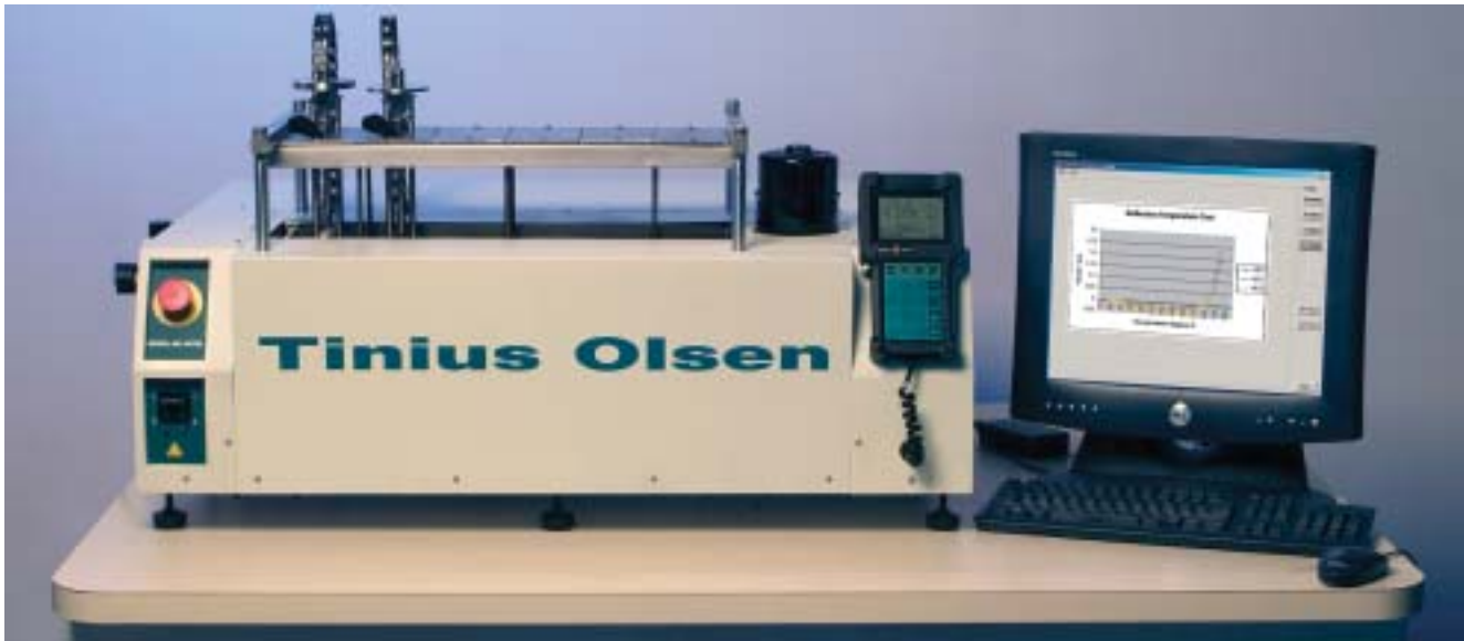
Fig 1. Model 603 HDTM shown with two test stations, one for deflection temperature and one for Vicat testing. The stations are raised for easy and rapid specimen insertion prior to a test and for specimen removal at the end of the test.
